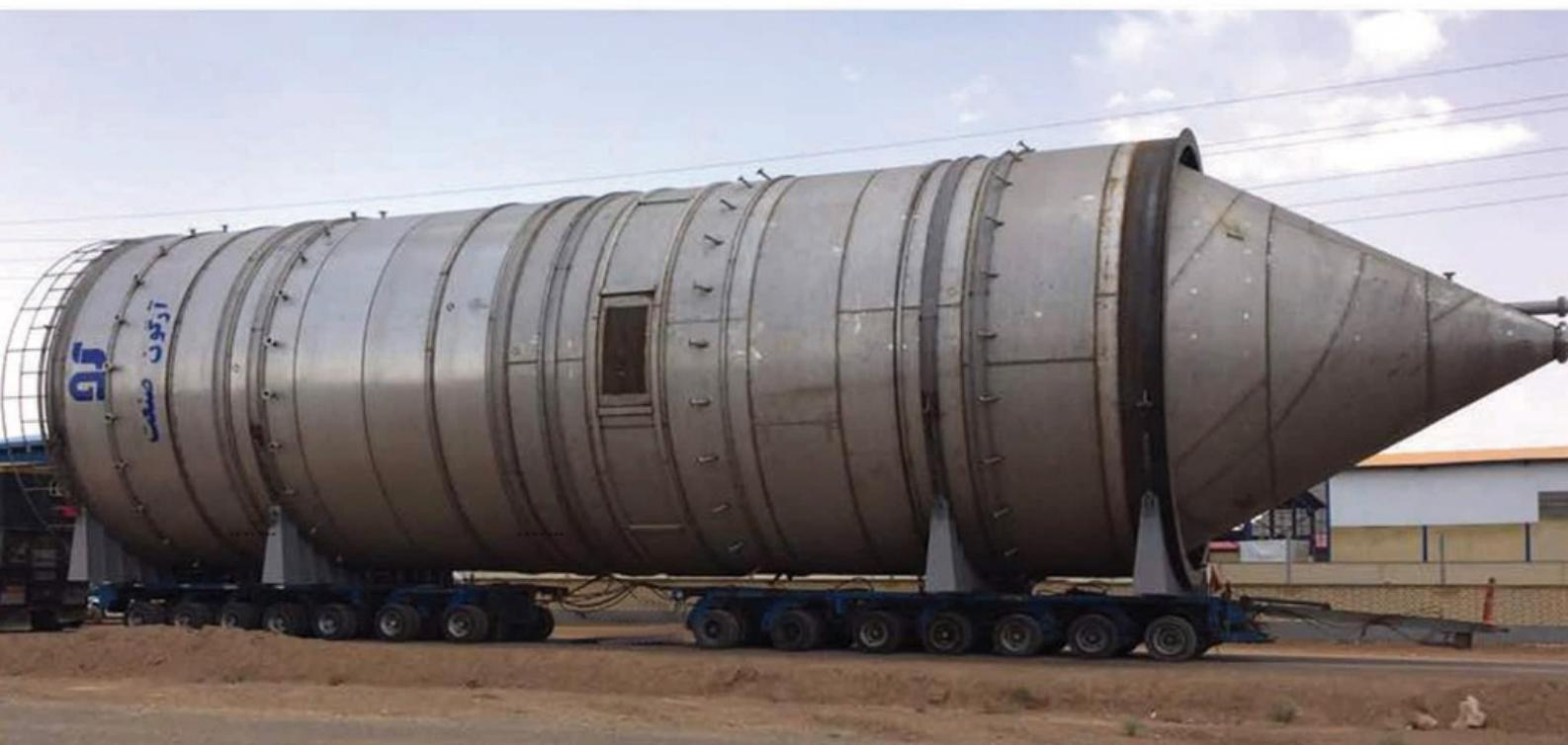
This tank designed, manufactured and developed by Argon Sanat company for the first time in the Middle East. It stands at a height of 32 meters, a diameter of about 8 meters and a capacity of 1,100,000 liters, which distinguishes it as the largest tank construction, outside of the consumer area in the country and the Middle East.
